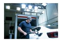
With the new fast charging system, charging processes can be tested under real climatic conditions in the MAHLE climatic wind tunnel.
